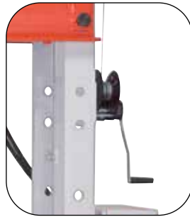
Winch provides easy positioning of press bed
